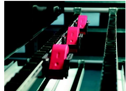
For rapid-moving items, several wireless sensors per shelf permit needs-based control of replenishment, for example at assembly workstations.
